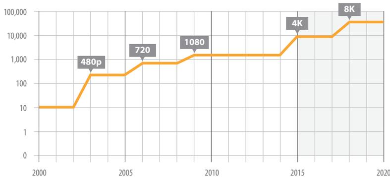
Each step corresponds with an increase of resolution: 480i, 480p, 720, 1080, and then projected bumps to 4K and 8K. Note that on this logarithmic graph, each step represents a roughly tenfold increase in file size. **Video is getting big.**
